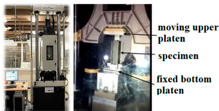
Figure 5. Zwick \pm 250 kN Fatigue (left) and Instron Drop Tower (right).
