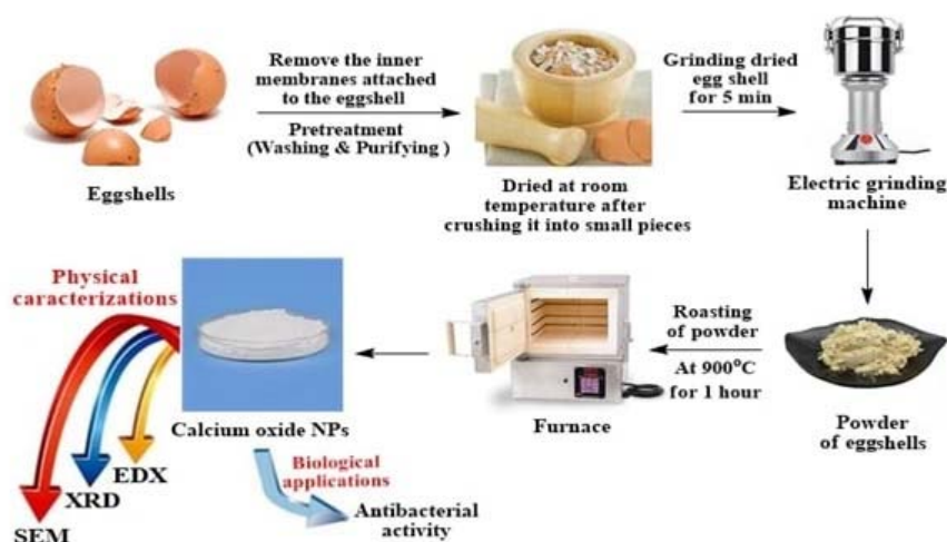
Figure 2. Diagram of preparation and applications of CaO NPs
