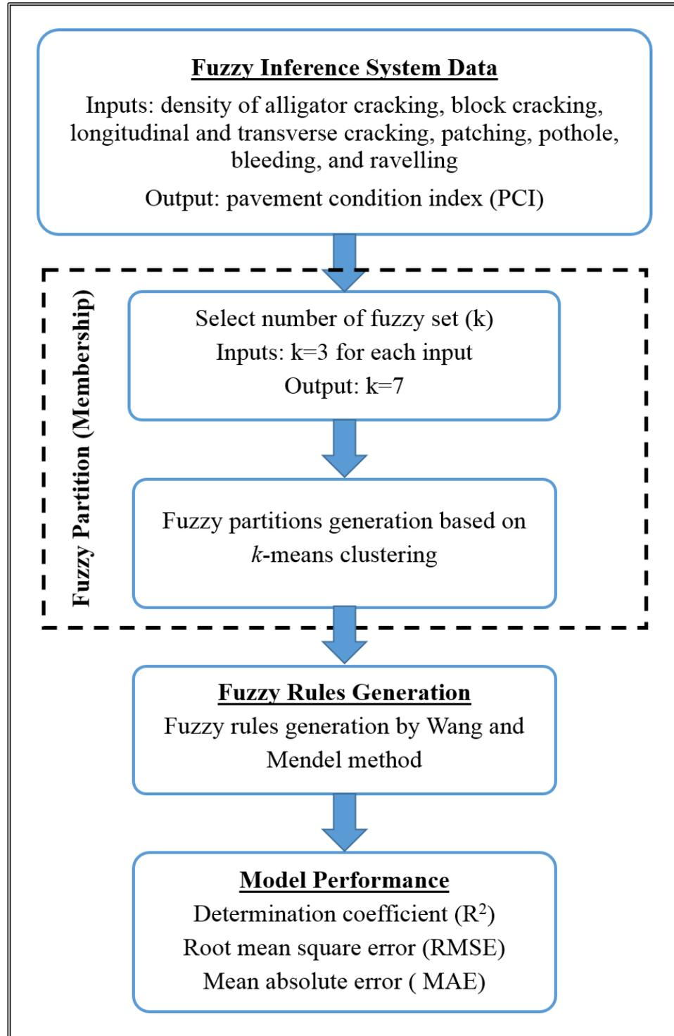
Figure 5-2: Flow chart of a pavement classification model based on FIS.
