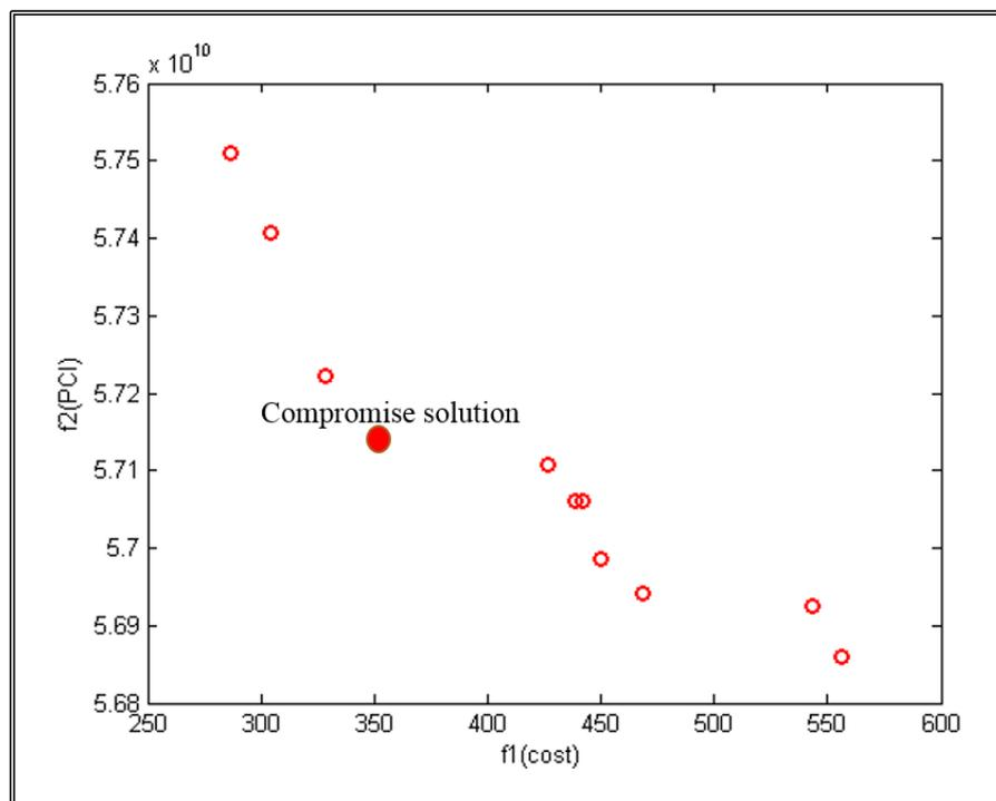
Figure 8-1: Non-dominated solutions and compromise solution after 10 iterations.
