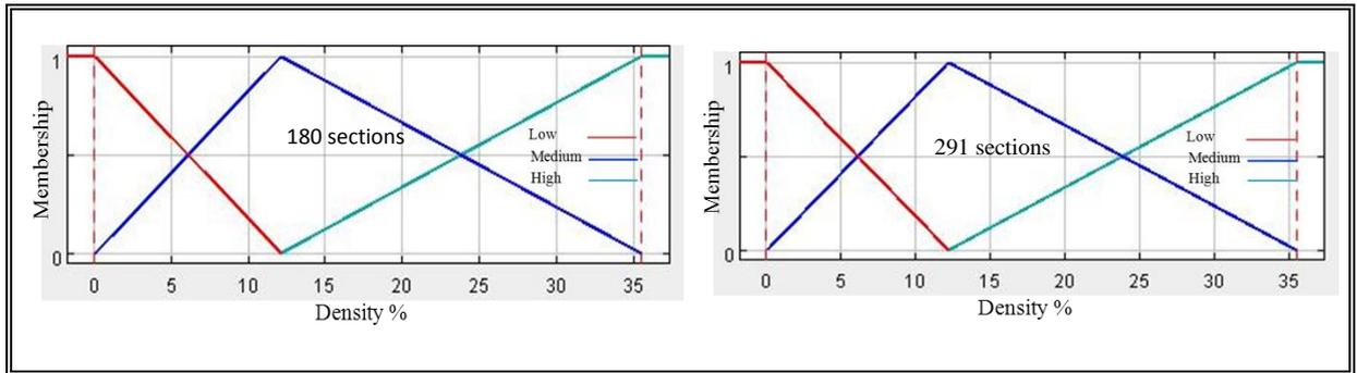
Figure 5-7: Membership functions for Patching.
