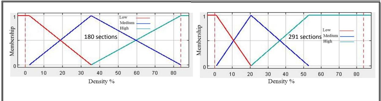
Figure 5-4: Membership functions for Alligator cracking.
