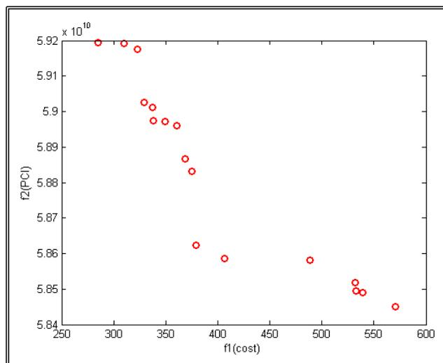
Figure 7-10: Non-dominated solutions of DMOPSO after 100 iterations.
