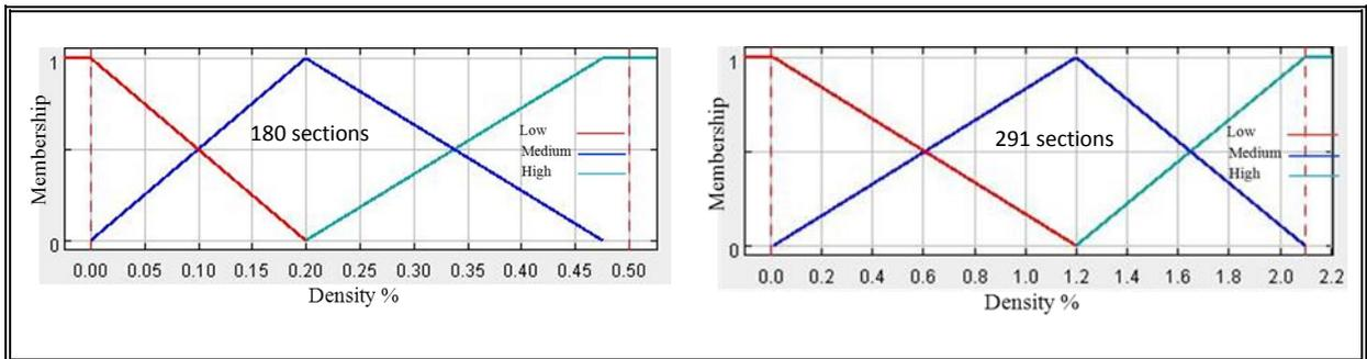
Figure 5-8: Membership functions for Potholes.
