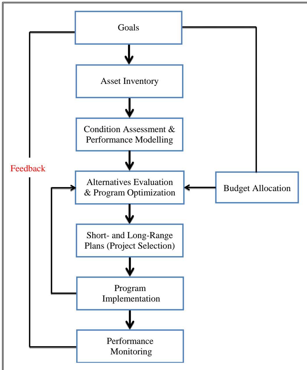
Figure 1-2: Specific components of typical asset management system (U.S. Department of Transportation, 1999).
