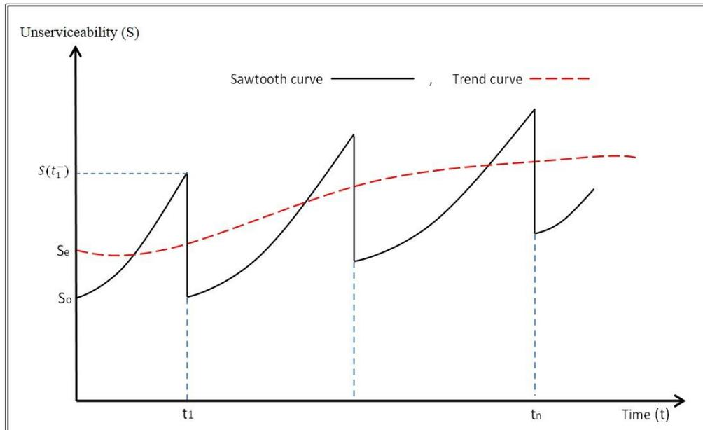
Figure 3-3: Sawtooth curve and trend curve of pavement serviceability (Tsunokawa and Schofer, 1994).
