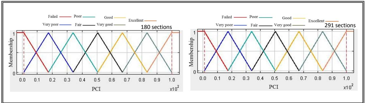
Figure 5-11: Membership functions for PCI.
