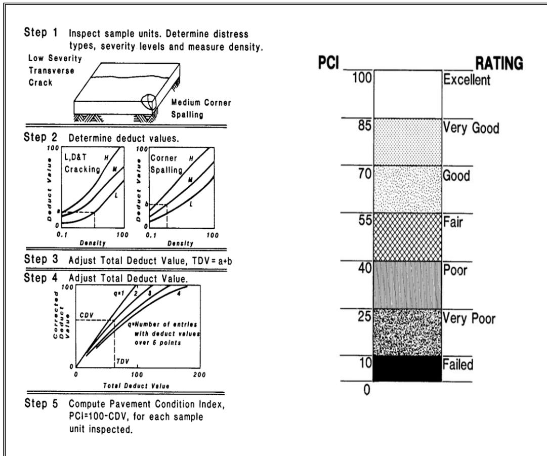
Figure 2-1: Pavement condition index (PCI) calculation procedure (Fwa, 2006).
