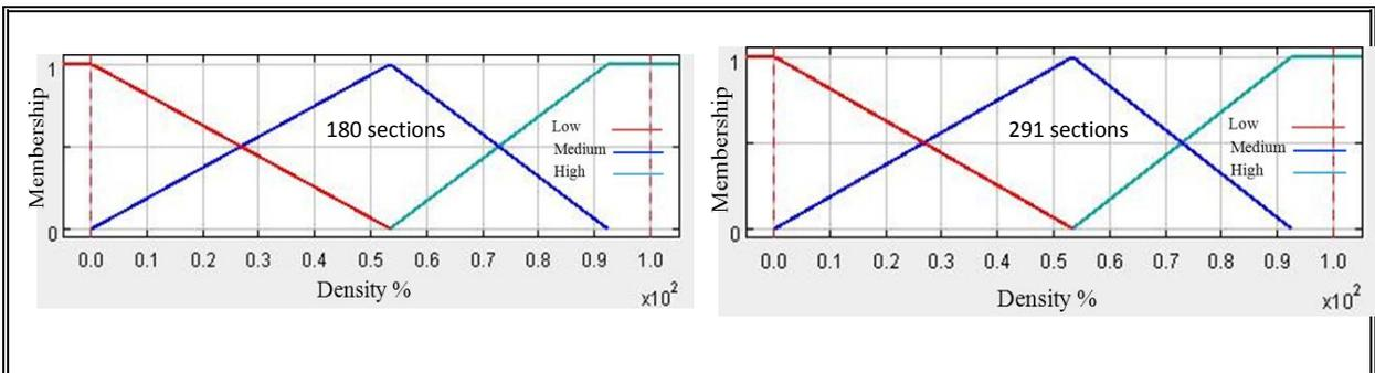
Figure 5-5: Membership functions for Block cracking.
