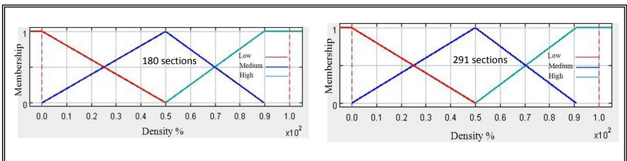
Figure 5-10: Membership functions for Ravelling.
