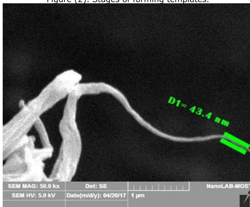
Figure (3). Scanning electronic microscopy of nanocellulose prepared from sugar cane residues
