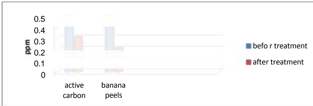
Figure 13. - Nickel treatment by banana peels comparing with active carbon.
