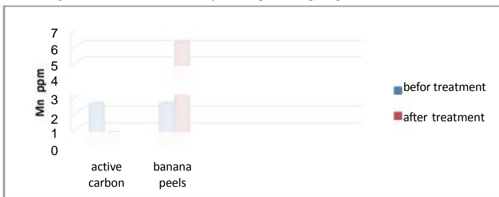
Figure 11. Manganese treatment by banana peels comparing with active carbon.
