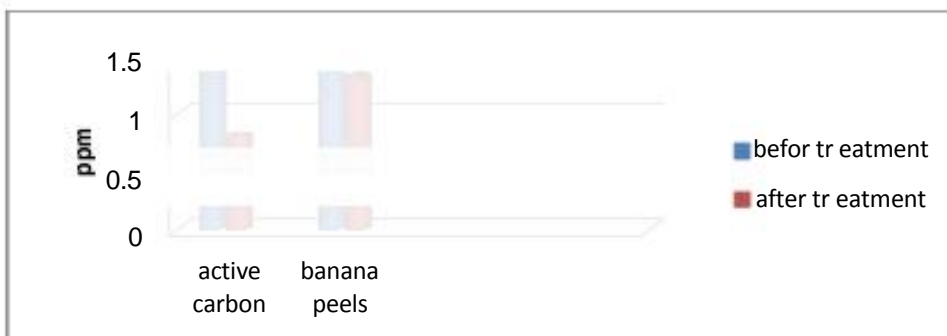
Figure 5. Total phosphate treatment by banana peels comparing with active carbon.
