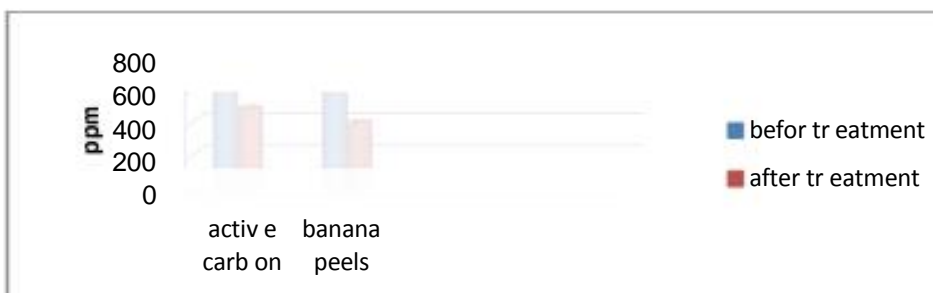
Figure 6. Total Magnesium treatment by banana peels comparing with active carbon.
