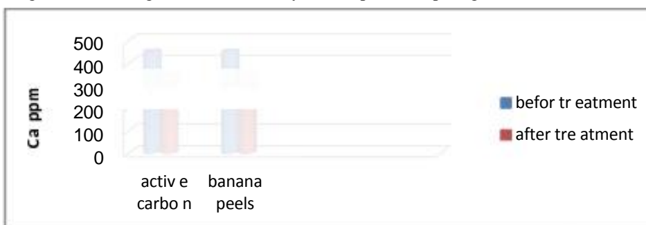
Figure 7. Total calcium treatment by banana peels comparing with active carbon.
