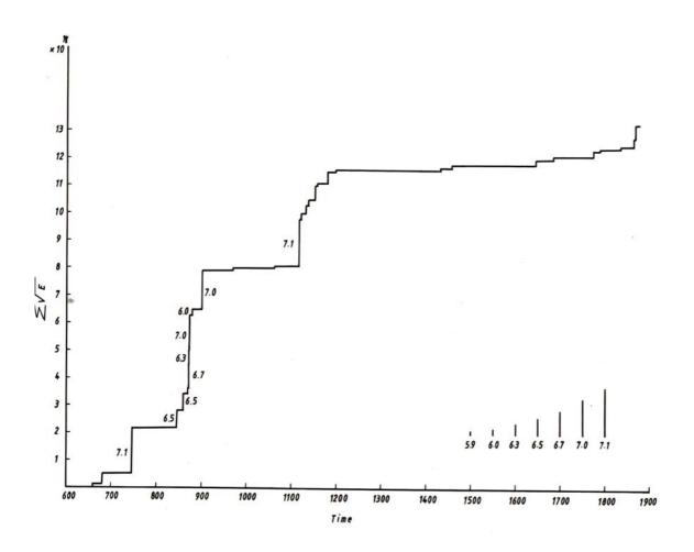
Figure (4) Cumulative Seismic Strain Release.
