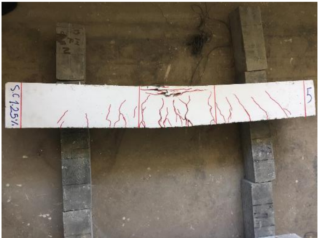
Figure 4-25 Crack patterns of beam SC1.25
