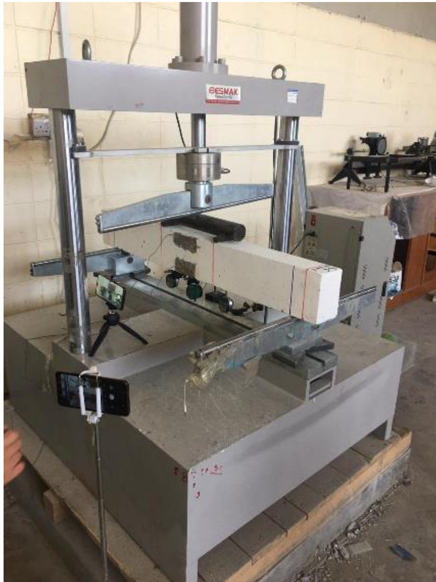
Figure 3-10 Experimental setup for flexural beams
