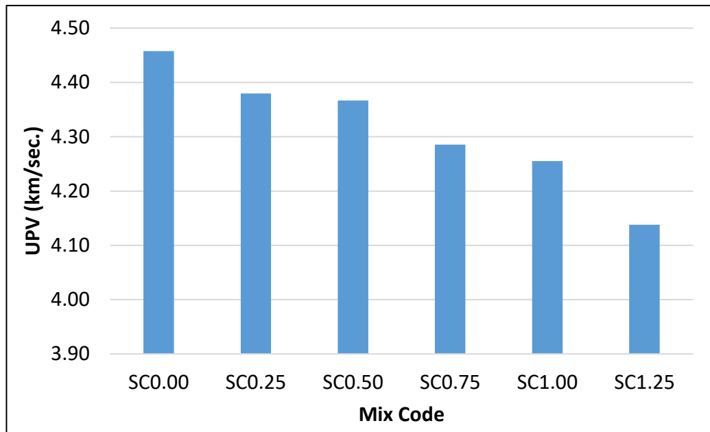
Figure 4-7 Ultrasonic pulse velocity (UPV) test results for all mixtures
