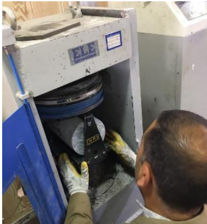
Figure 3-7 Splitting tensile strength test setup
