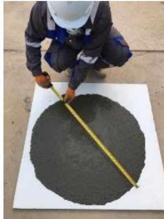
Figure 3-4 Slump flow test setup
