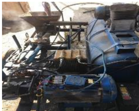
(c) Shotcrete body
