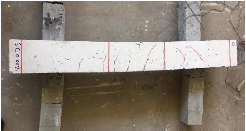
Figure 4-20 Crack patterns of beam SC0.00
