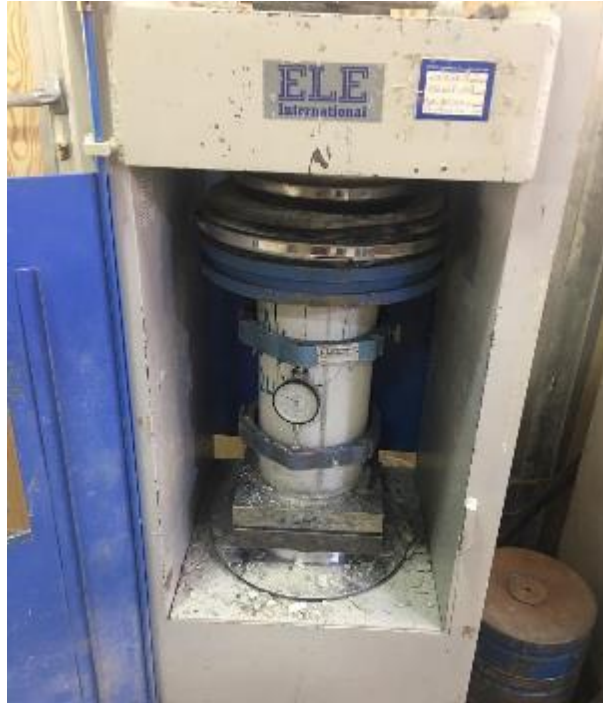
Figure 3-8 Modulus of elasticity test setup
