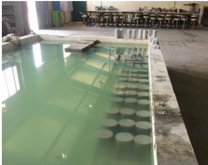
Figure 3-3 Curing process of shotcrete samples
