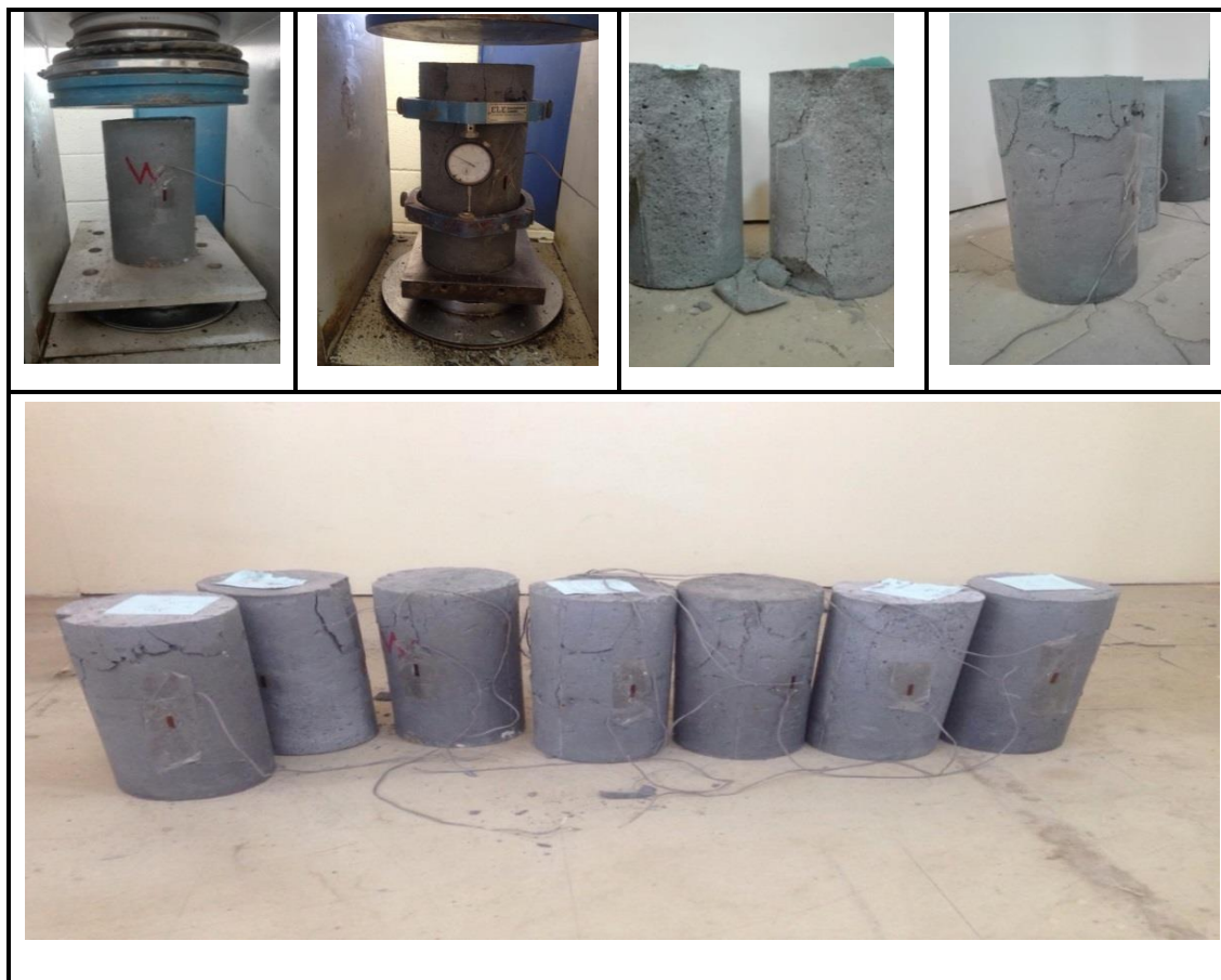
Plate 4-5: Shape of failure of all investigated mixes.
