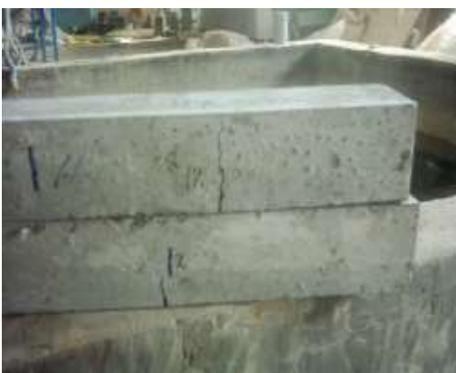
Plate (4-2) The mode of failure of specimens after testing
