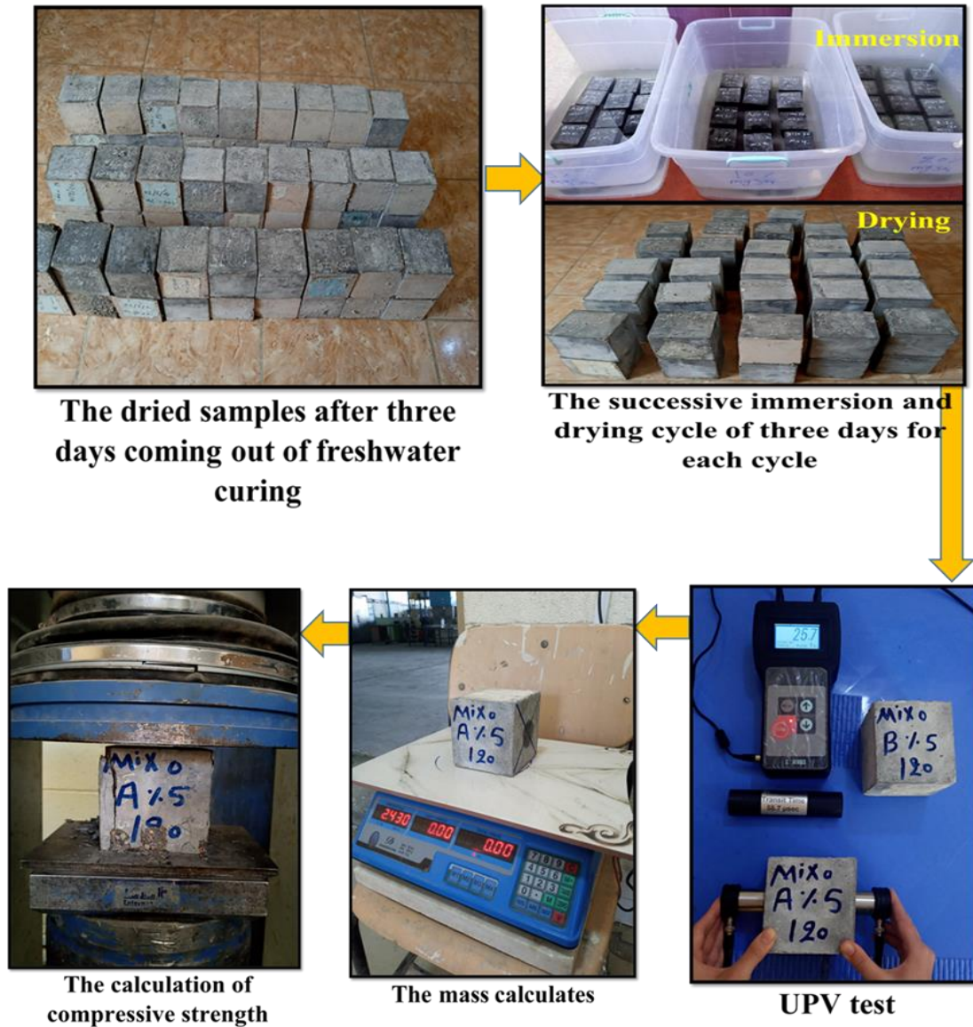
Figure (3-52): Treatment and test process for the samples immersed in magnesium sulfate solution
