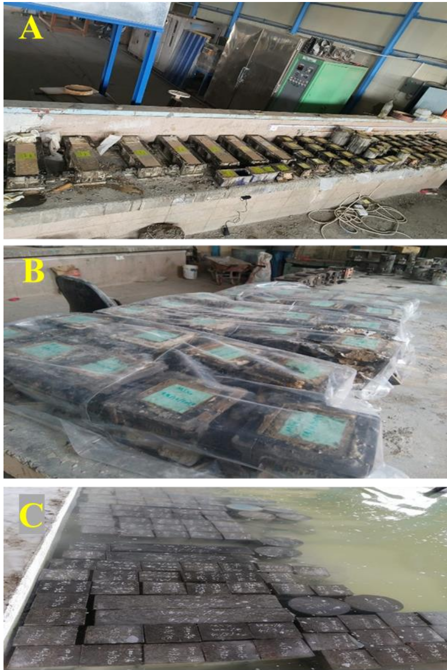
Figure (3-38): [A] Casting of samples, [B] Covered of samples with polyethylene sheets, [C] Curing of samples.
