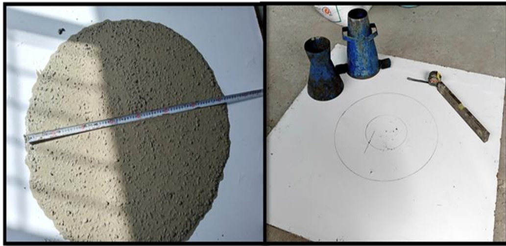
Figure (3-39): Slump flow test for SCC
