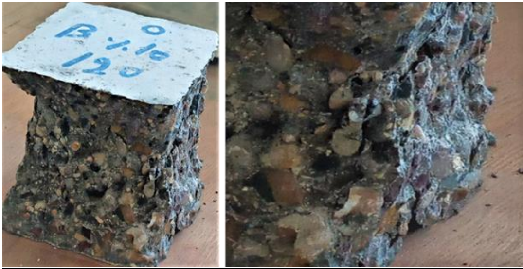
Figure (4-46): Sample of control mix (SCC0) after immersion cycles wet and dry in 10% MgSO_4 solution at 120 days.
