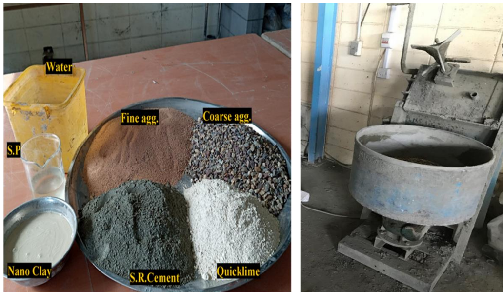
Figure (3-37): Mixing materials and concrete mixer.
