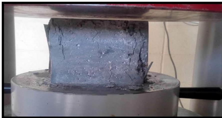
Figure (3-47): Compressive strength test for SCCs
