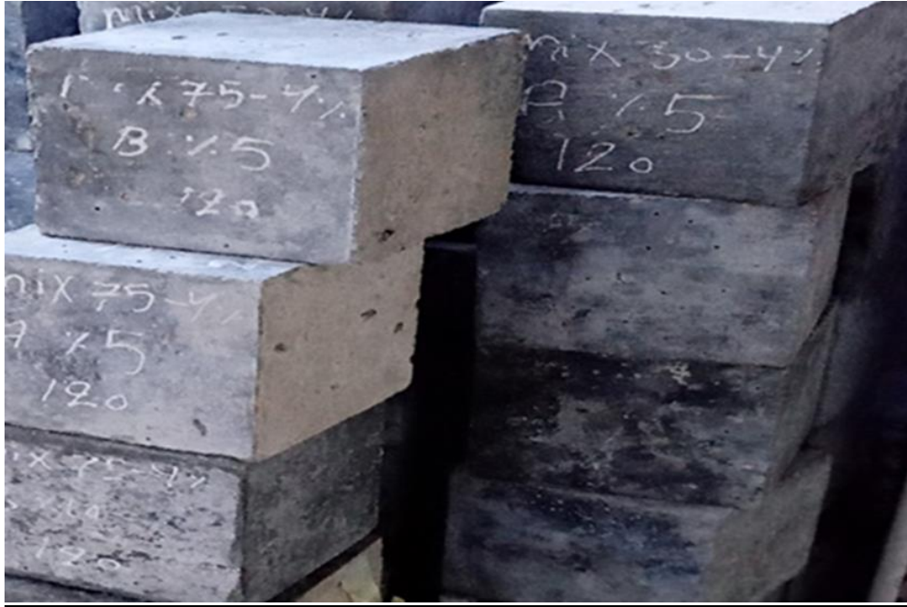
Figure (4-36): Specimens exposed to magnesium sulfate attack
