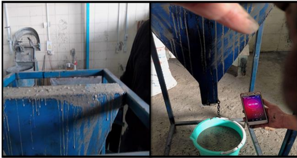
Figure (3-40): V-funnel test for SCC.
