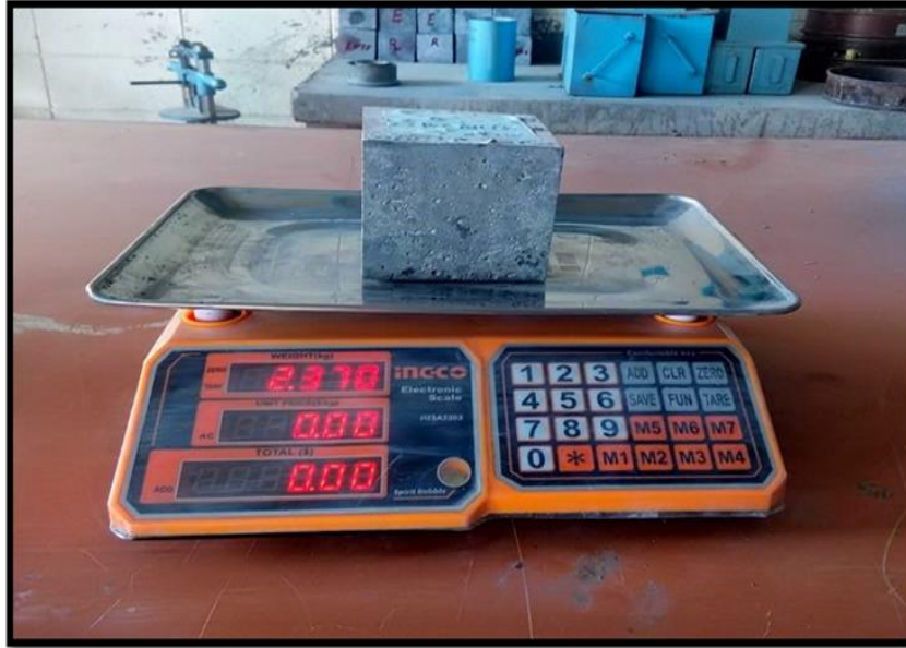
Figure (3-45): Dry density test for SCCs
