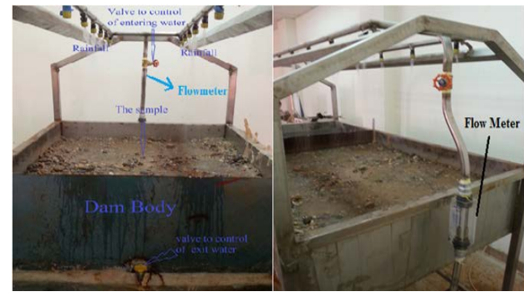
Fig. 3 the model of Sand Storage Dam
