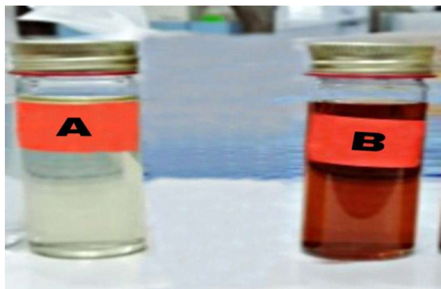
Fig. 1. Color change of AgNO 3 (pale-yellow to brown color) denoting the synthesis of AgNPs
