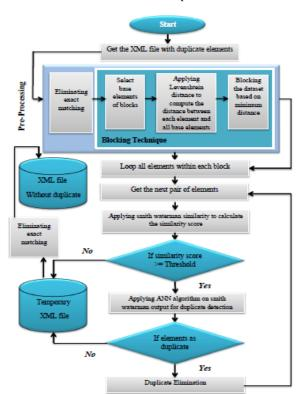
Fig. 4: Flowchart for Proposed Work.
