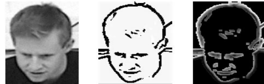
Figure 1: Detected edge and image subtraction
