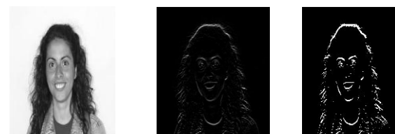
Grey scaled image, Image with vertical filter, Binary image
