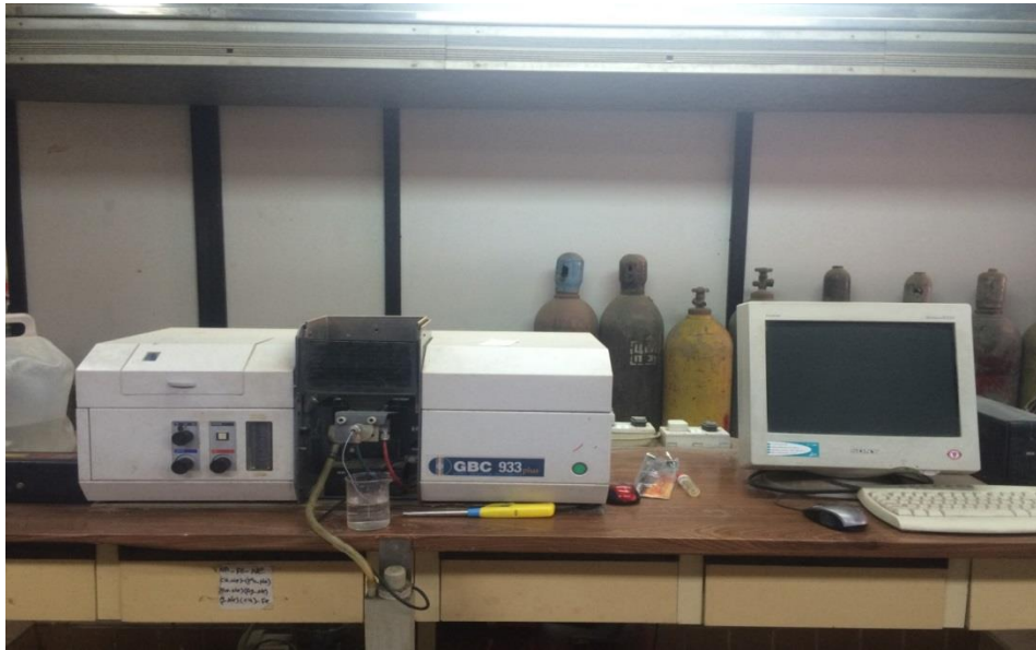
Figure 2. Atomic Absorption Spectrometer
