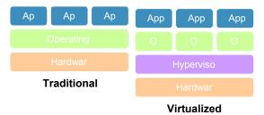
Figure 6. Traditional and Virtualized stack
