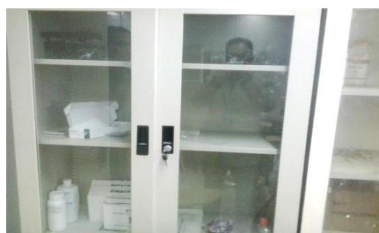
Figure 6: No information regarding the chemicals stored in the cupboard.
