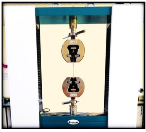
Figure 2. Shows the device used in the tensile testing process
