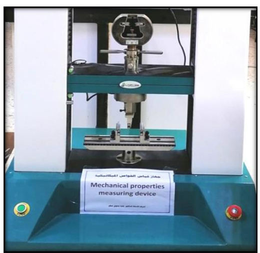
Figure 6. LAREE device used in conducting bending tests
