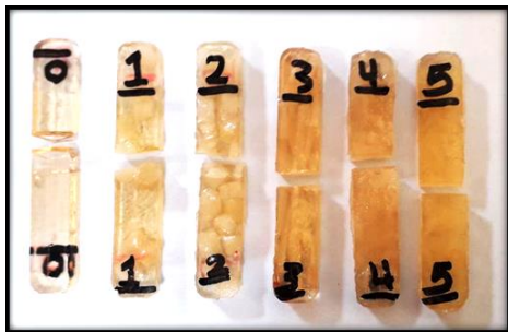
Figure 8. Bending test samples after conducting mechanical tests
