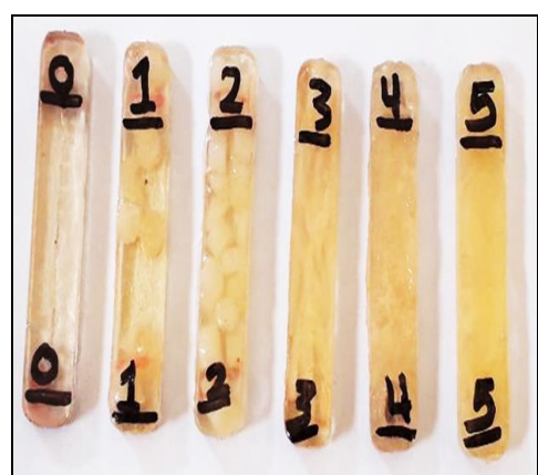
Figure 7. Bending test samples before carrying out mechanical tests.
