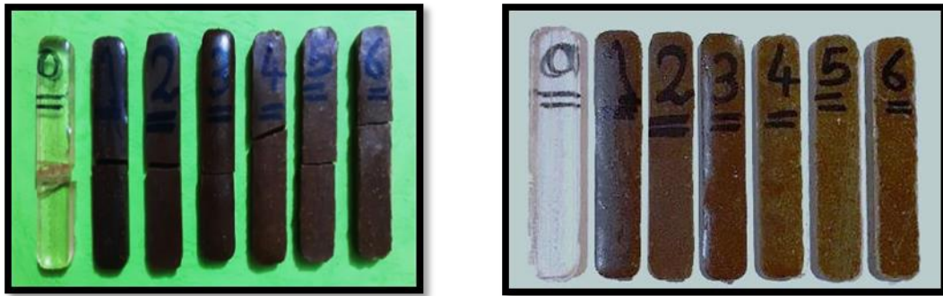
Figure (3-b) Shock resistance test samples before and after the test.
