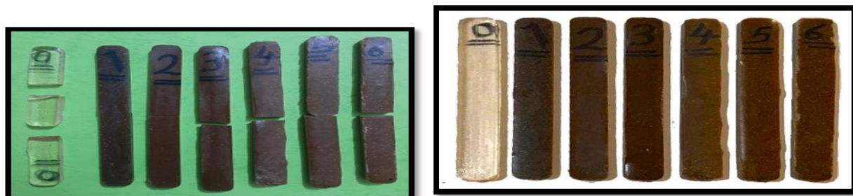
Figure (4-b) Bending resistance test samples before and after the test.
