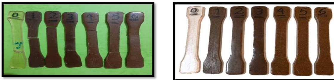
Figure (1-b) Tensile strength test samples before and after examination.
