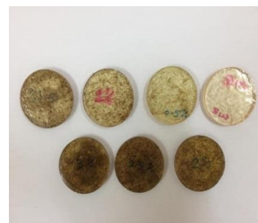
Figure (3). Dimensions of the hardness test samples. Figure (4). Samples used in hardness test.
