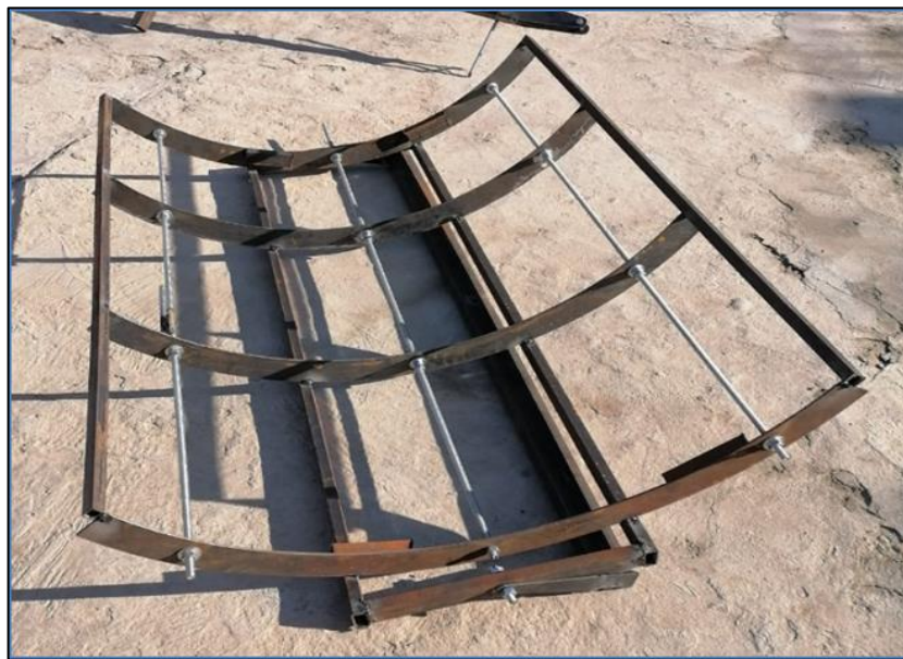
Figure 3.3: Frame structure of the reflector
