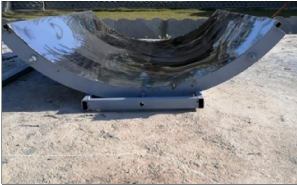
Figure 3.4: Reflective surface structure
