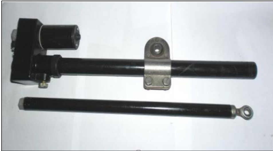
Figure 3.8: Electric motor for tracking.
