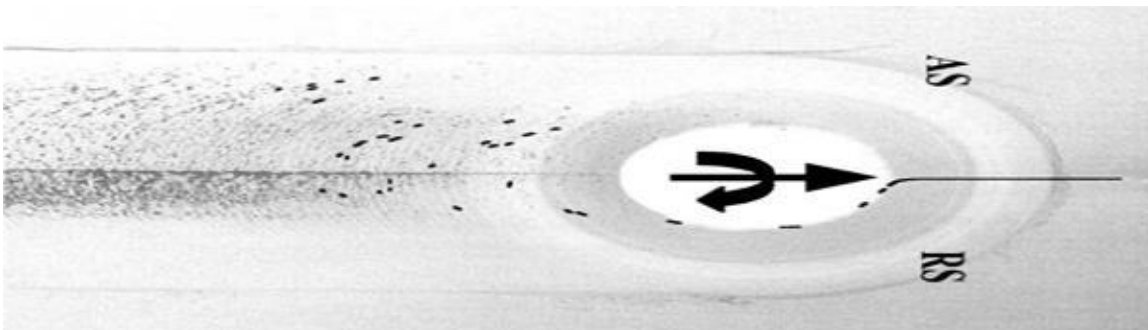
Figure (1.4): Advance and Retreating sides for weldment [16].
