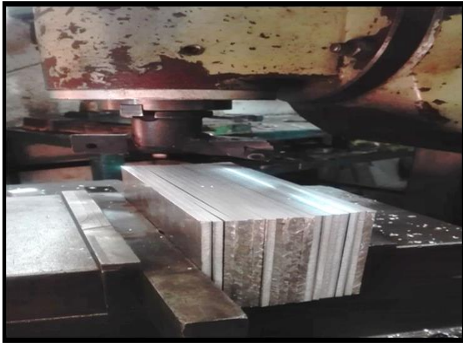
Figure (4.6): Preparation plates before welding operation.
