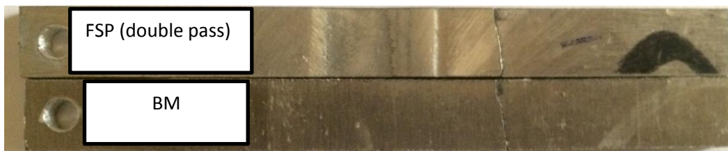
Figure (5.22) fatigue fracture location for BM and double pass (at low stress level).
