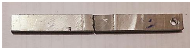
Figure (5.20): Fatigue fracture location for single pass.
