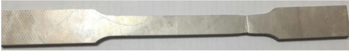
Figure (5.1): Orientation fracture for the base material.
