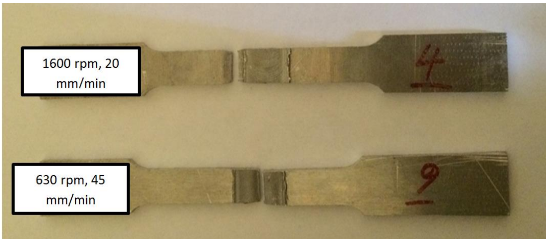
Figure (5.5): Orientation fracture for (90°).
