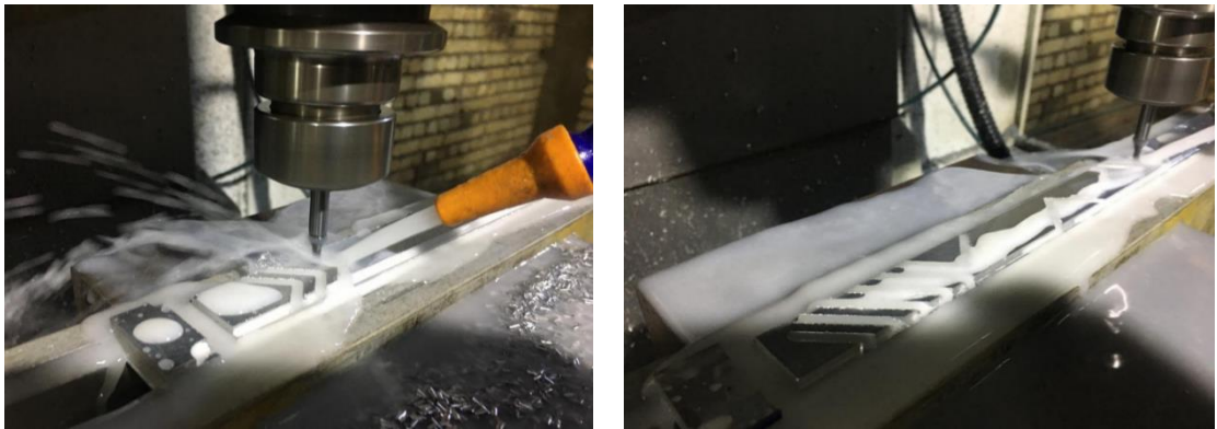
Figure 4.3: Photographs illustrate the forming process of the grooved channel on the bottom wall of the channel by using CNC machining.
