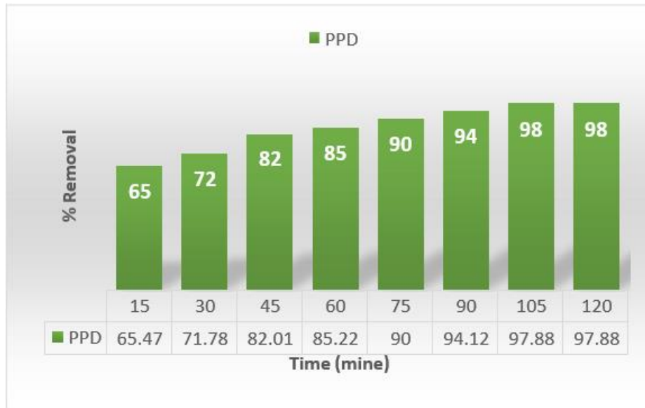
Figure (8): Effect of contact time of adsorption of tincture (PPD) on (CdO -NPs)
