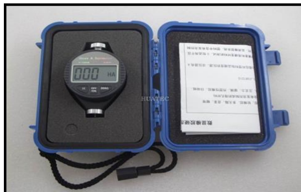
Figure 7. The hardness measuring device
