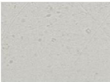
Figure 16: PVC Contain 0.4% ZnCl 2 after Irradiation
