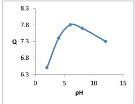
Fig. 9: Effect of the acidity function on the adsorption capacity of the nickel ion  $Ni^{2+}$  by P.H.A
