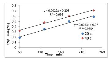
Fig. 11-a: Adsorption kinetics of nickel ion Ni<sup>2+</sup> mediated by poly(styrene-co-methyl metha acrylate) hydroxamic acid at temperatures 20  $^{\circ}$ C , 40  $^{\circ}$ C
