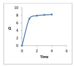
Fig. 8: The effect of time on the sorption capacity of the nickel ion  $\mathrm{Ni}^{2+}$  by P.H.A .
