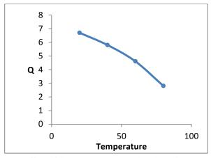
Fig. 10: Effect of the Temperature on the adsorption capacity of the nickel ion Ni<sup>2+</sup> by P.H.A
