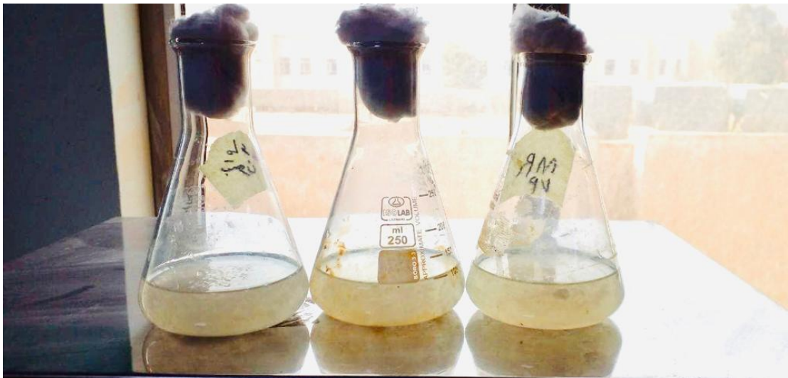
Figure 5 shows the effect of incubation duration on plastic decomposition Figure (6) Biodegradation of plastic underoptimal PH7, temperature 30 °C, vaccine volume 1 ml, incubation duration of 21 days)
