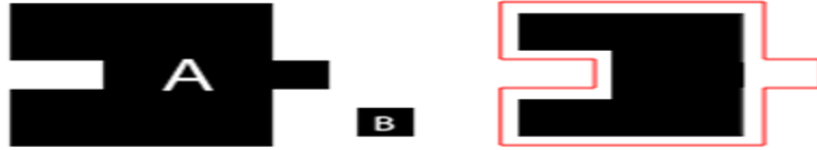
Figure( 2.16) Binary Erosion of an Image A by a Structuring Element B[31].
