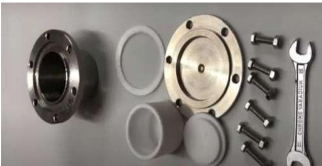
Figure 2.1: Hydrothermal autoclave reactor.
