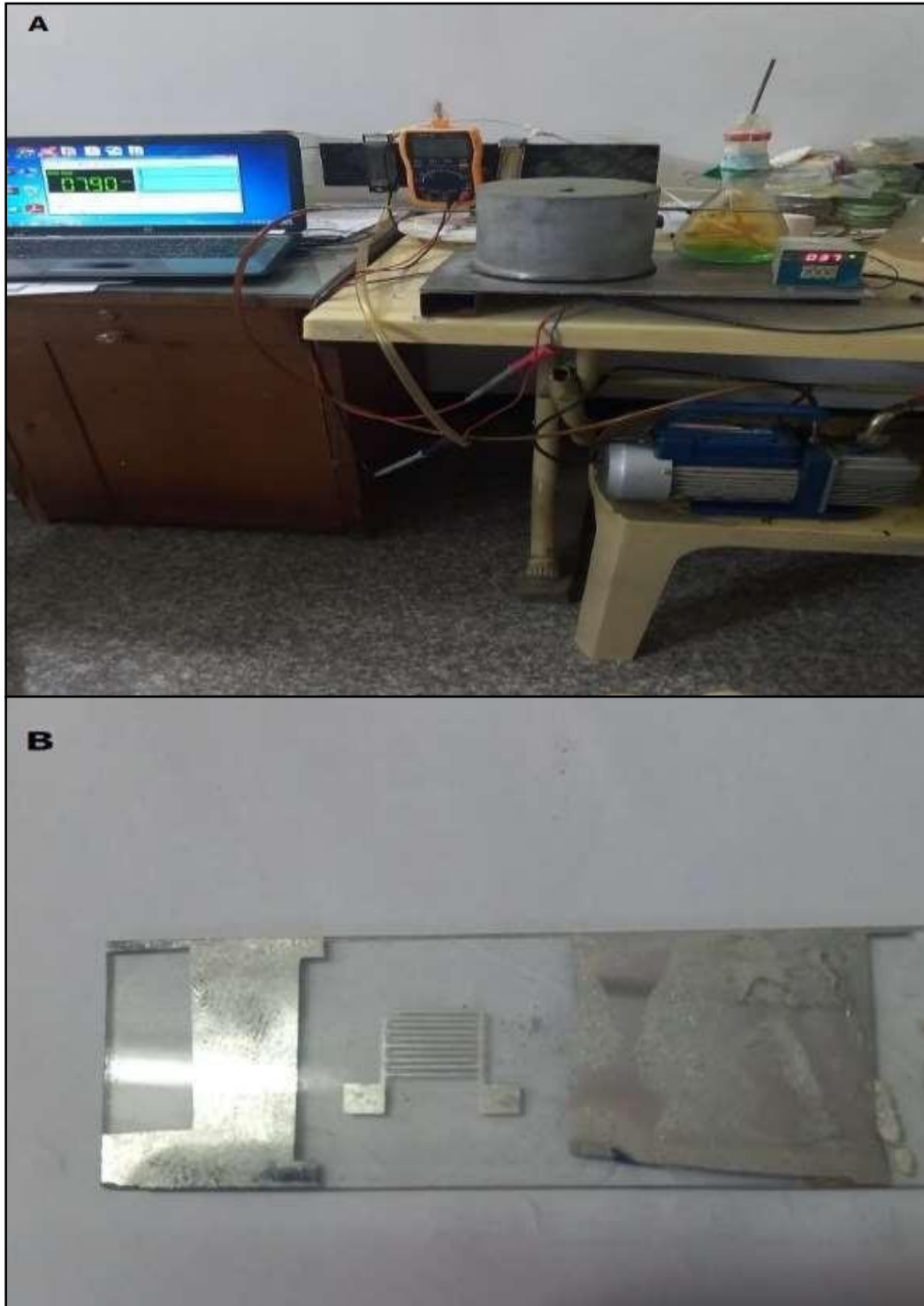
Figure 2.3: (A) Gas sensor testing system; (B) Gas sensor sample setup.
