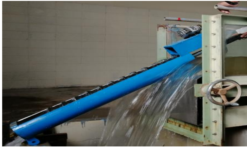
Fig. 4. Archimedes screw after completion of manufacturing
