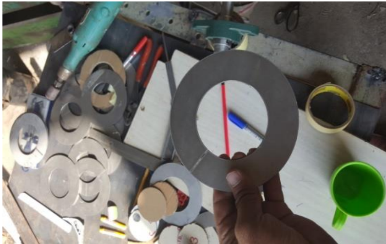
Fig. 2. The helix before welded on shaft
