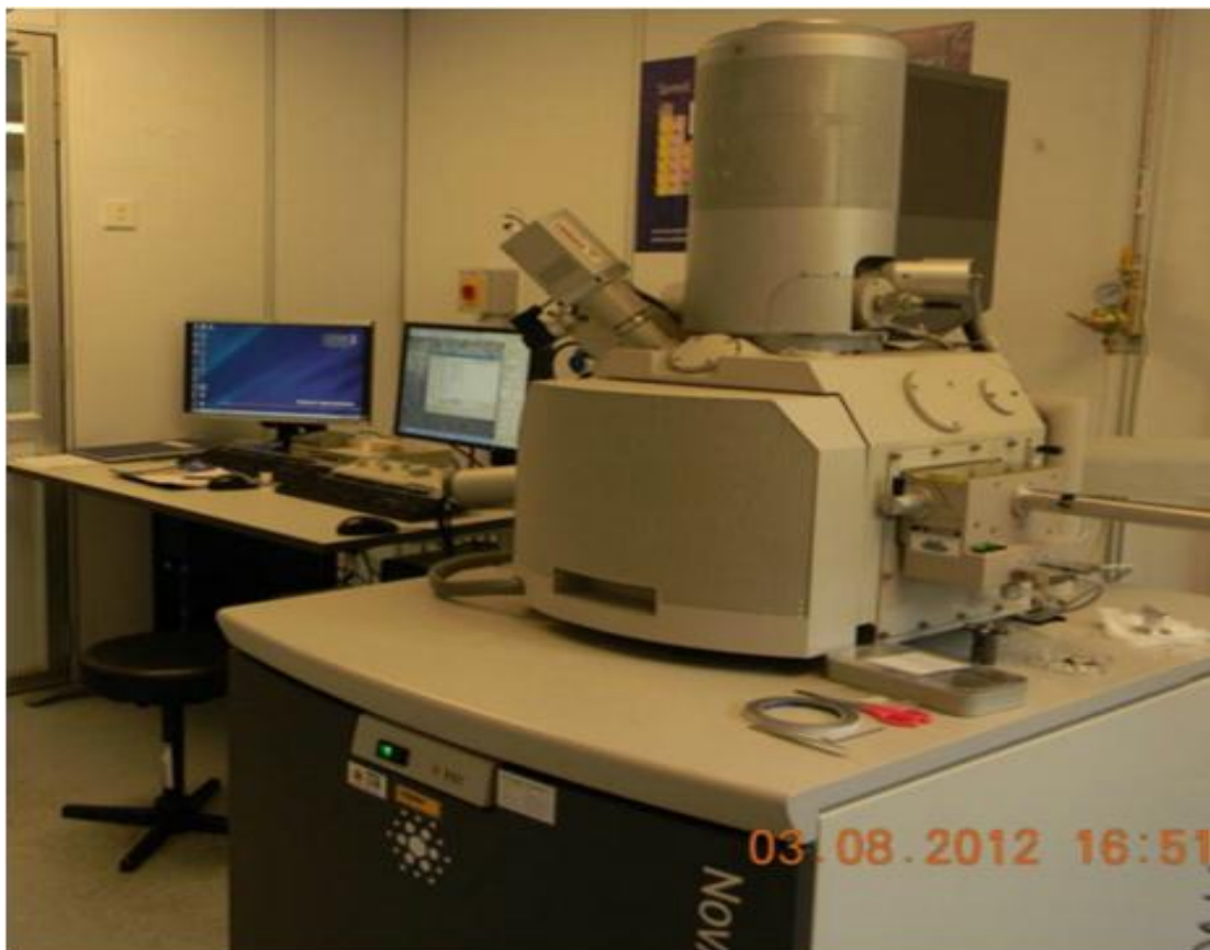
Image (2-3): Field emission scanning electron microscopy system
