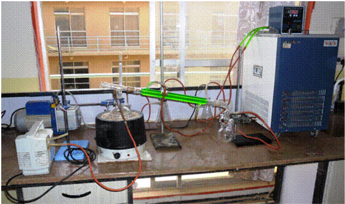
Image (2-1): Apparatus used in vacuum distillation for the preparation of carbon from heavy fuel oil residues
