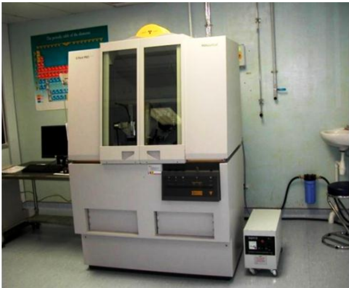
Image (2-5): High resolution X-ray diffraction equipment
