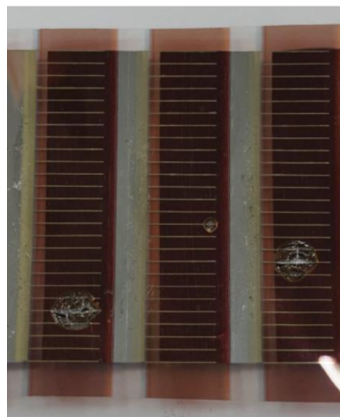
Fig. 6. The picture illustrates critical failure of devices during switching seen as burn and/or melted areas of the organic solar cell.
