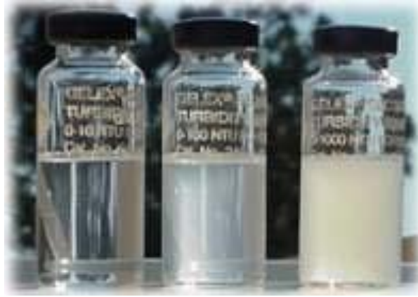
Photo (2-1) Turbidity standards of 5, 50, and 500 NTU [25]
