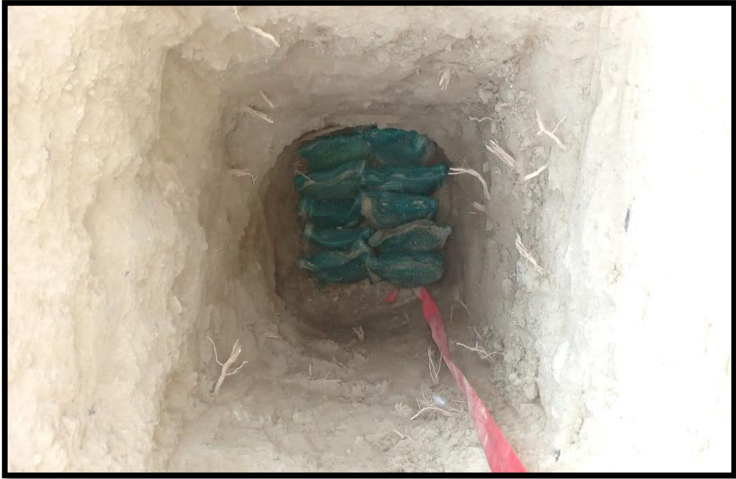
Figure2.6: Place the samples inside the hole.
