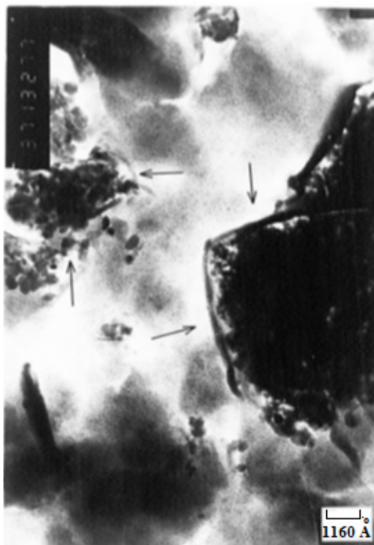
Figure 9 Transmission electron micrograph of Sn(IV)TPPCl 2 adsorbed on montmorillonite surface. The appearance of the complex is indicated by the arrows.
