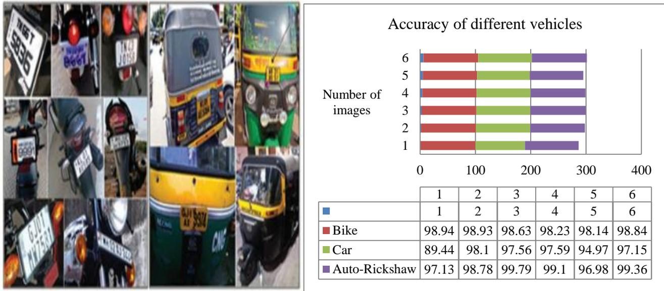
Fig. 10 Images of various vehicle types and their accuracy in recognition
