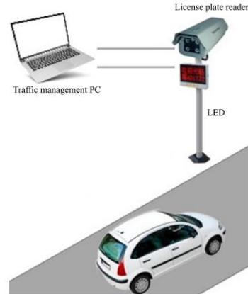
Fig. 1 Car number plate detection overview
